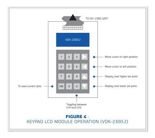
Keypad/LCD Board can be hot plugged/removed to/from Actuator Controller Board. Actuator Controller Board can detect when Keypad/LCD Board is plugged in and then activate LCD display with following text:
