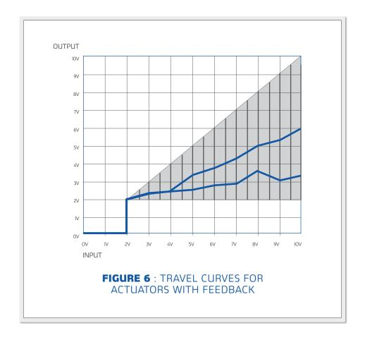
With FEEDBACK "ON" (SW-2) operation only, values in the shaded zone can be programmed
